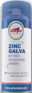
**ZINC GALVA aerosol is a zinc-rich primer/paint designed to protect surfaces from corrosion. Zinc Galva works by providing a sacrificial zinc rich film which by electrolytic action prevents corrosion of underlying steelwork. Suitable for use as a primer coating Zinc Galva may be over painted where required. Galva is particularly effective in the protection of galvanised surfaces and steelwork following cutting and welding.**
